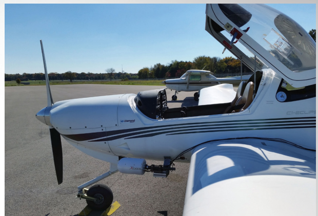
The small plane used for data acquisition with the WaldoAir XCAM-B mounted underneath
